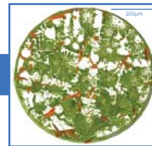
3D volume slice of an AlMg5Si7 alloy ( \varnothing 350 \mu m): Fe-aluminides and Mg 2 Si-phases.
