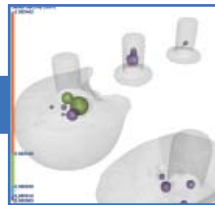
nanoCT ® of TSVs in an electronic package. The voids in the copper filling are clearly visible.
