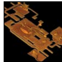
3D Computed Tomography of a ceramic SMD IC
