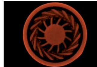
Sintered micro turbine ( \varnothing 3 \text{ mm} )
