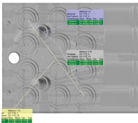
Top view of the valve block with three distance measurements.
