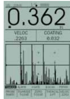
A-scan with display of coating layer and material wall thickness
