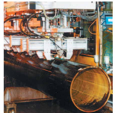
Weld seam inspection on SA-longitudinally welded pipes
