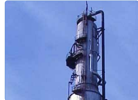
Crude Unit Overheads may suffer severe corrosion due to crude slate changes/treatment misapplications but require significant mobilization preparation for inspection
