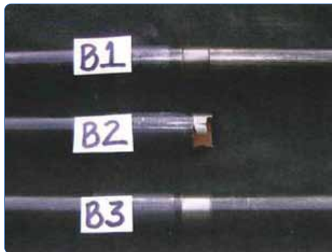
Heat exchanger tubing can suffer specific damage that can be precisely qualified by ET
