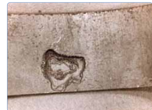
MIC can be highly localized and cause penetration in a short period of time
