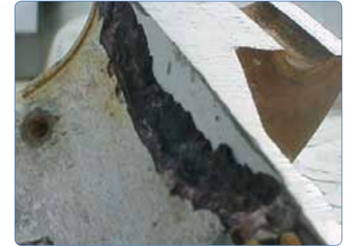
HF scale and corrosion can significantly compromise flange integrity
