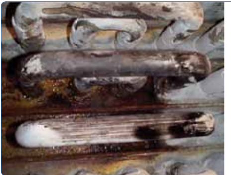
Crude Unit Convection Cross-Over's may suffer severe corrosion due to crude slate changes to higher TAN Crudes
