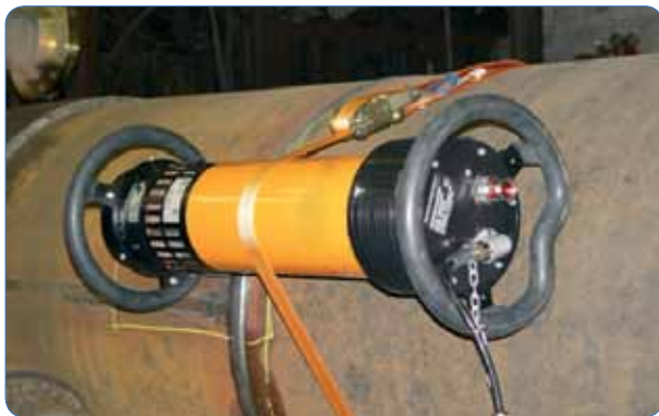
Field portable ERESKO X-ray generators are used for a wide variety of film, CR and DR corrosion detection and sizing applications.
