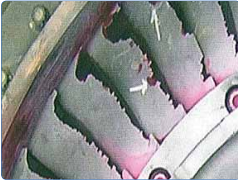
Catalyst and solid can cause severe damage to rotating and stationary blades
