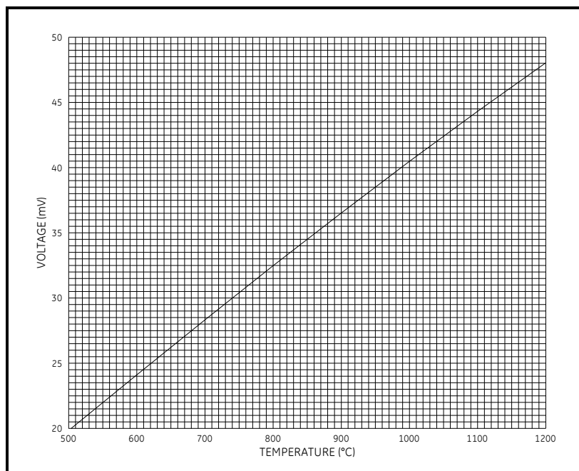
Figure 28: Thermocouple Voltage vs. Temperature
