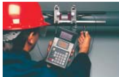
Technician using Panametrics PT868 portable meter to monitor flow on a 4 inch line.
